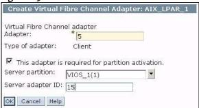
Create the second Virtual FC Client Adapter with the slot number details as shown the <u>figure 2.6</u>. Make sure the slot numbers match with the slot numbers we have entered in the second VIOS LPAR while creating the Virtual FC Server Adapter.
