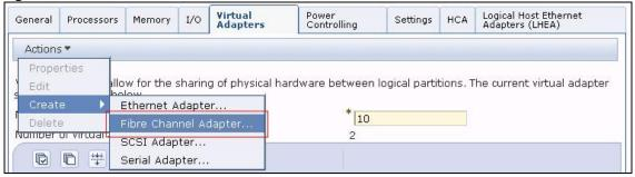
Input the first Virtual FC Client Adapter slot number details as shown in the <u>figure 2.5</u>. You need to make sure that the slot numbers entered is exactly matching with the slot numbers entered while creating the Virtual FC Server Adapter in the first VIOS LPAR. This adapter will be the first path for the SAN access in the AIX LPAR.
