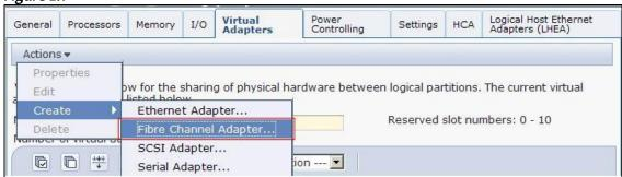
Input the Virtual FC Server Adapter slot number, select the client LPAR from the dropdown which will be connected to this server adapter and input its planned Virtual FC Client Adapter slot number as shown in figure 2.2
