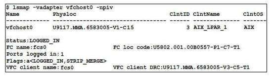
You can use the 'lsmap -vadapter vfchost0 -npiv' command. You can see that the port is logged into the SAN fabric and it shows the client LPAR details too.
